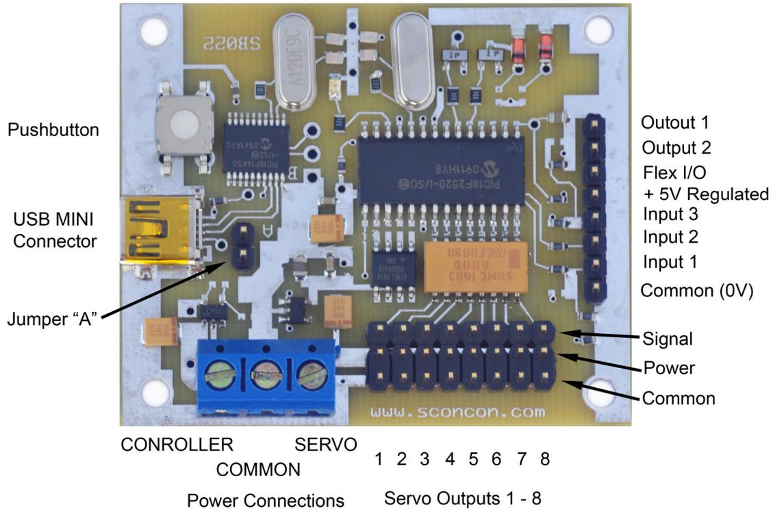
Recommended controller power is 5.5 - 12 Volts DC
